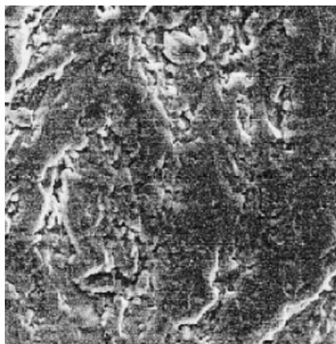
Fig. 2. The surface of the graphite, which was in contact with TEXTOR plasma, taken by SEM at normal incidence of e-beam. The picture frame is 60 × 60 μm.
